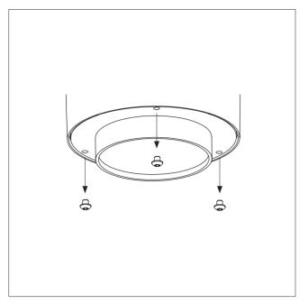
Unmount the current ring placed under the camera head by unassembling the three screws using the supplied tool.
