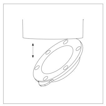
Position the lens and lens ring under the camera head so that the magnetic lens ring and the steel ring are connected correctly.
